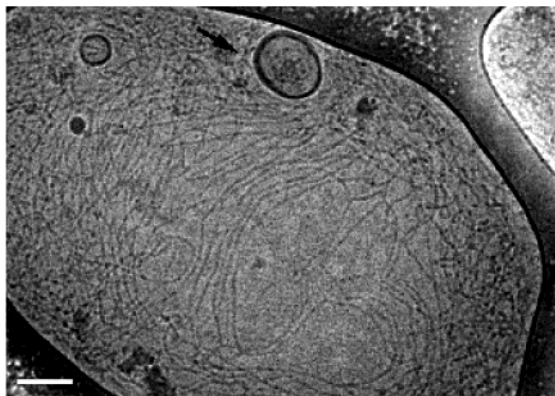
Figure 2. Cryo-TEM image recorded after a reaction time of 210 s for cationic templated silica. The arrow indicates a vesicular cationic surfactant-silica structure. Bar = 100 nm.
